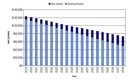
Figure 11: Projected Depreciated Replacement Cost
