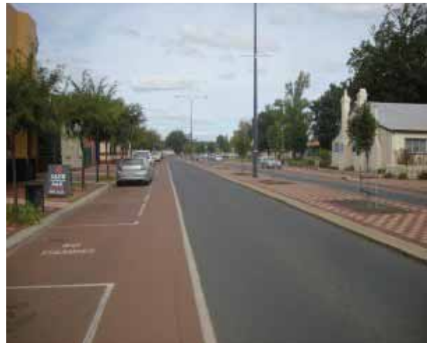
The main street of Donnybrook has been the subject of a streetscape improvement. The design of that street included provision of a 'bike lane' for cyclists as an integral component of the plan. The recent main street improvement in Toodyay did not provide such a facility.
