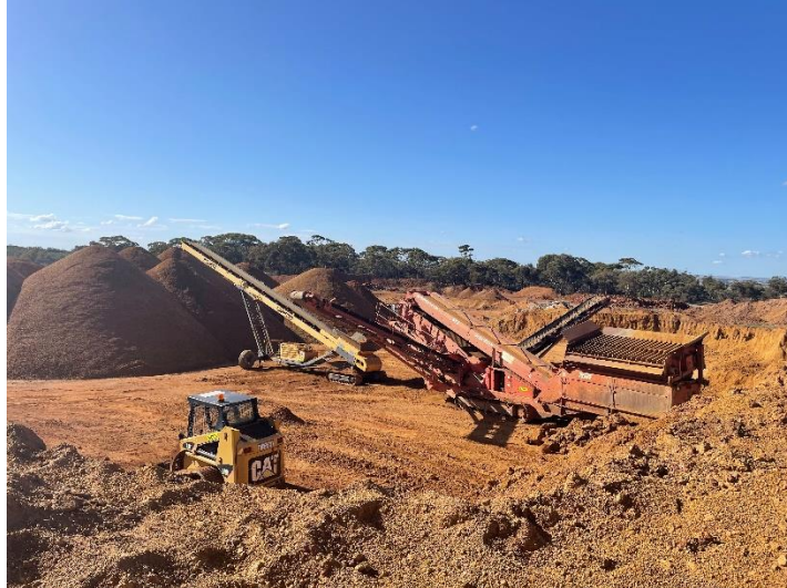
Photograph 9 – Current Operation of Pit with Screener/Crusher
