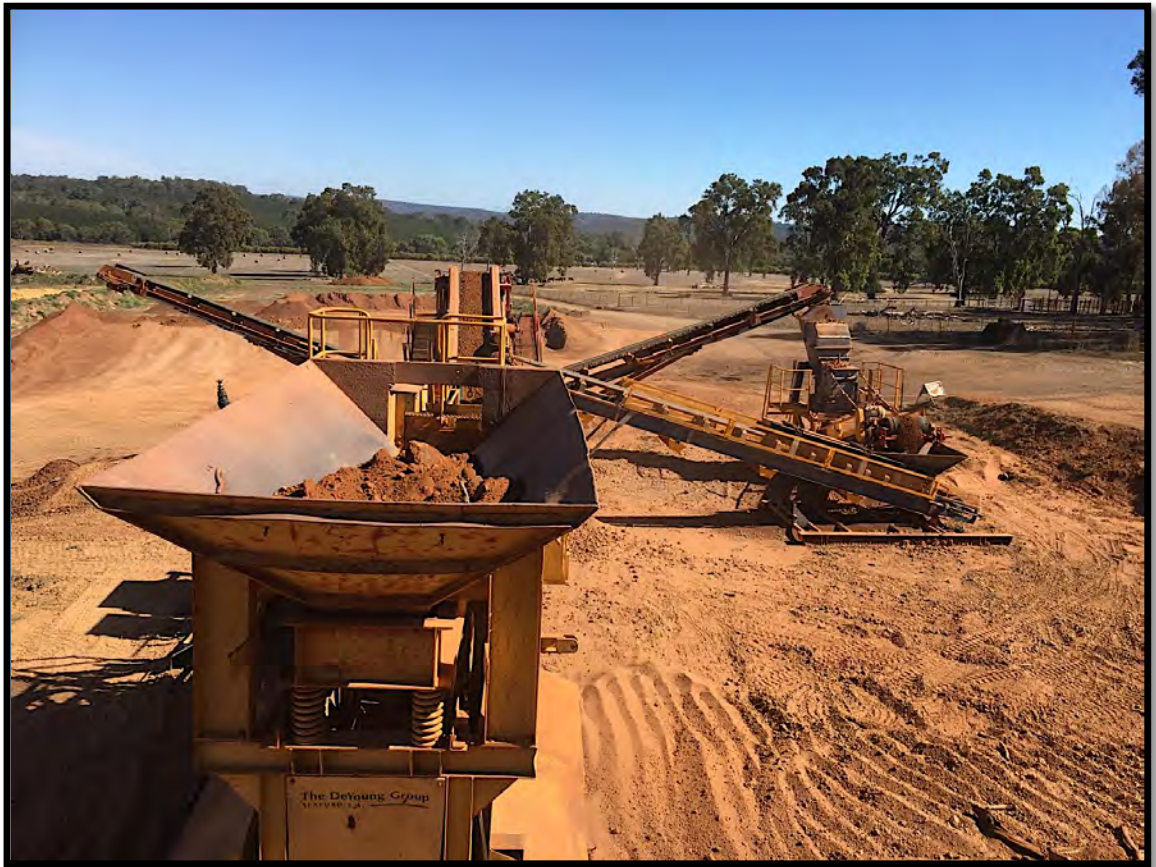
Figure B 1 Crushing laterite duricrust in summer. Note the lack of dust with the gravel staying moist into summer.
