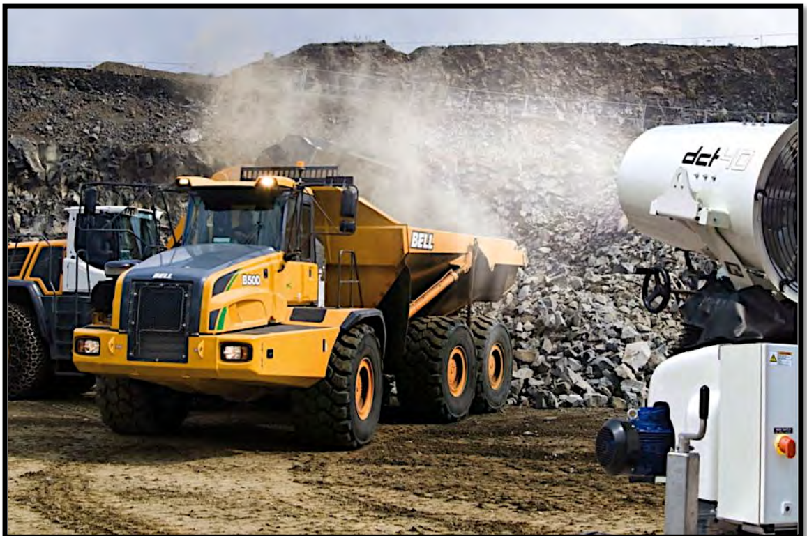
Figure B 4 A large mister used to capture dust during loading. A similar result can be achieved by wetting the rock prior to loading with a water canon.
