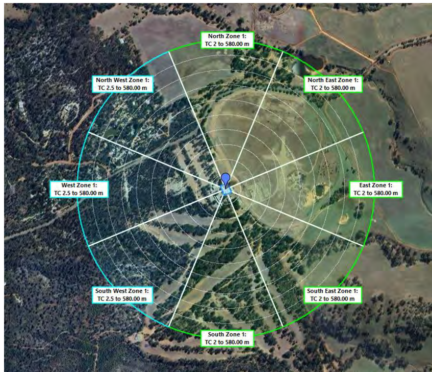
SATELLITE VIEW OF EXPOSURE OF STRUCTURE
